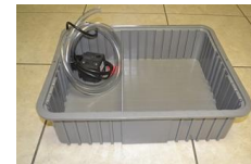
Tank and pump
